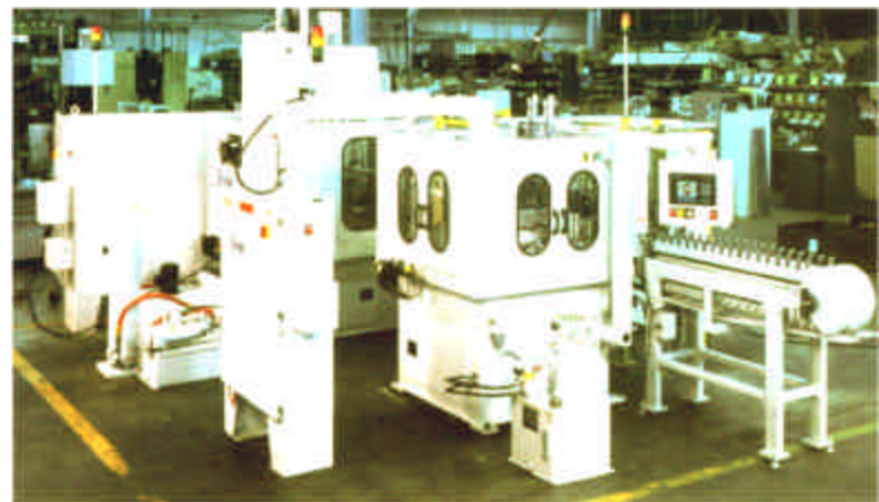
This Engis solution combines multiple machining operations – bushing Assembly, pad brushing, bore finishing, seat polishing and part washing – Into one end-to-end automated system.
