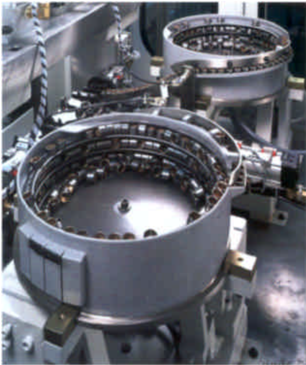
In this application, bowl feeders drop bushings into place, where they are automatically inserted into castings. Pick-and-place units transfer the castings into and out of the station.
