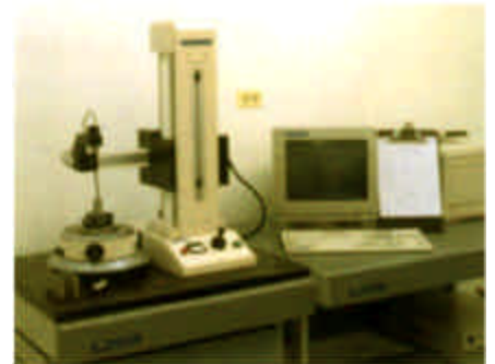
Prototypes and test-bed parts undergo rigorous inspection, utilizing the lab's computerized Talyrond system (above) and other devices to measure bore quality.
